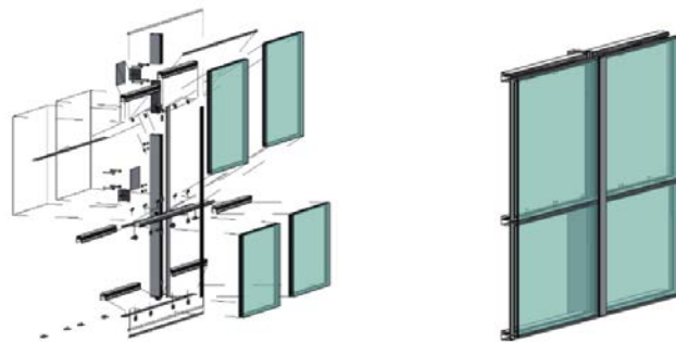
Fig.2 Installation Demonstration of Curtain Wall
